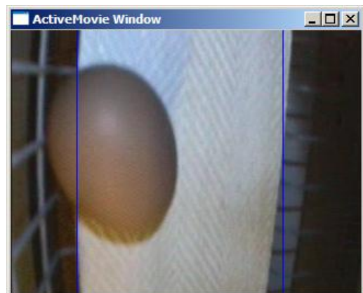
Figure 17. Image of an egg on the egg belt with vertical blue lines that show the extents of the belt material detected by the software.
