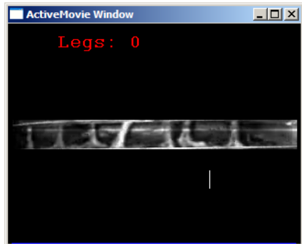
Figure 13. An example image displaying the search space for the leg scan algorithm.
