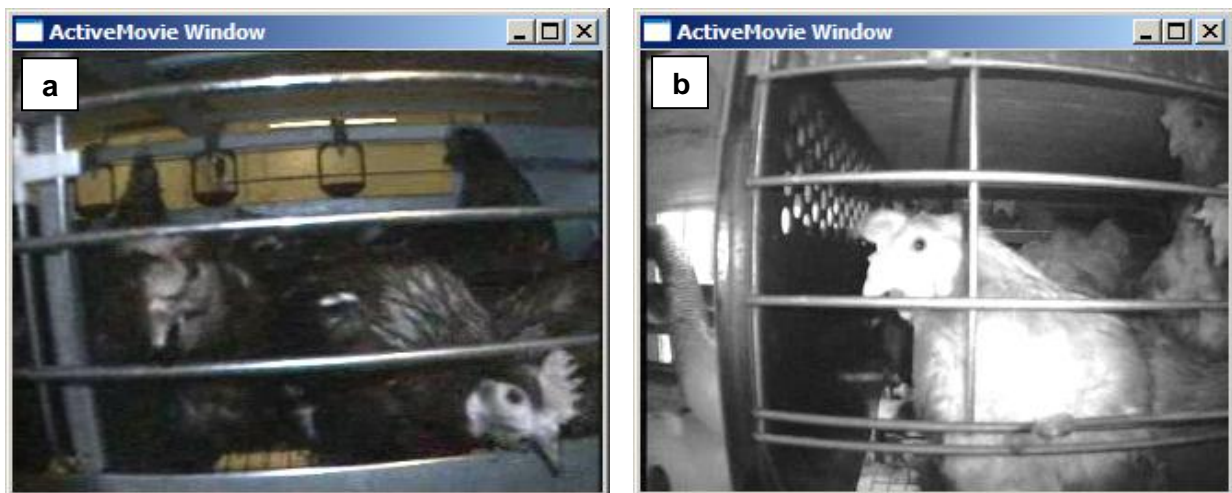
Figures 7a and b. Colour and infra-red images of hens in cages illustrating the eye of hens as a potential target for image recognition and tracking using video image analysis to count hens.
