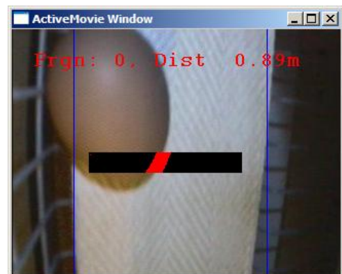
Figure 23. Image showing an egg entering the object detection area.
