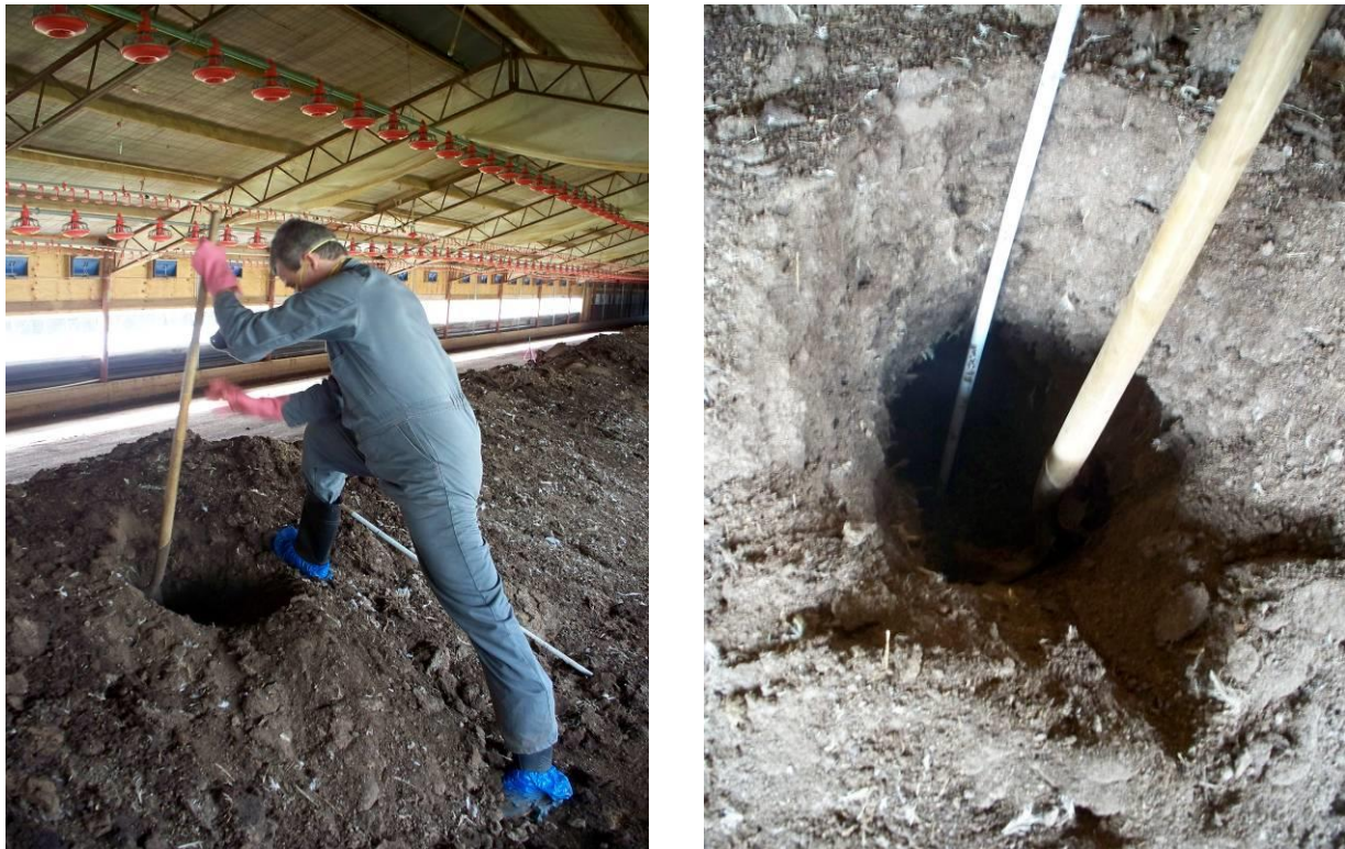
Figure 4-4: Litter collection from various depths of windrows
