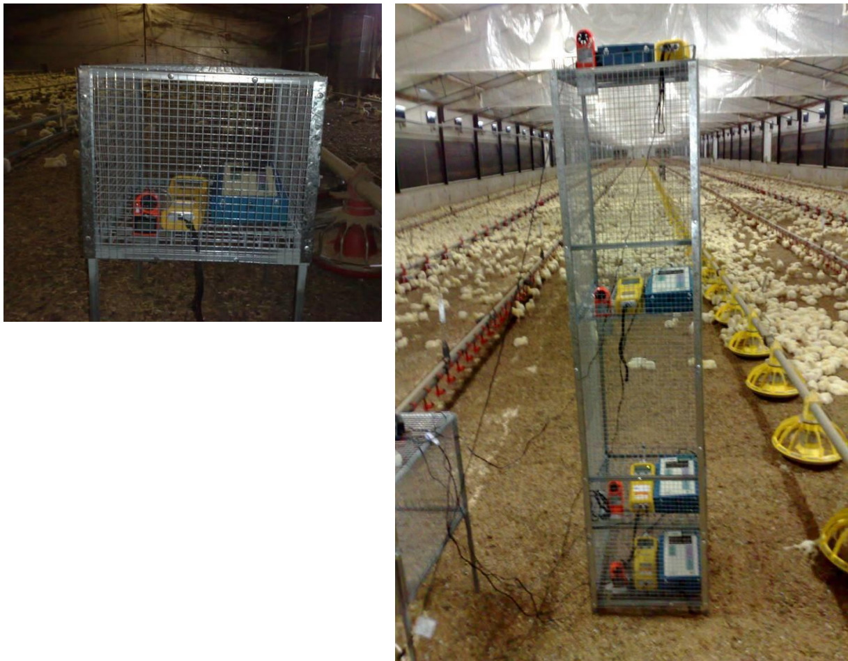
Figure 5-3: Custom made cage for placing three instruments at 30 cm ( left ) or at 5 , 30, 90 and 150 cm above the ground ( right )
