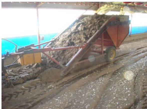
Figure 3-3: De-caking machine used to remove caked litter from the shed after removing birds and before heaping
