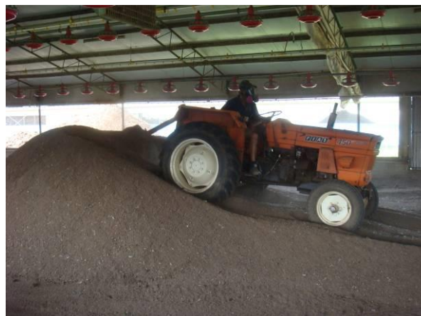
Figure 3-4: Using a tractor mounted blade to form the litter into heaps within the broiler shed
