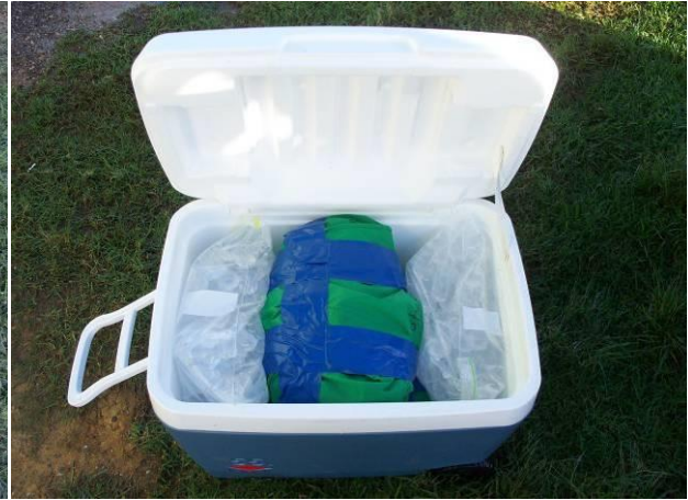
Figure 1-11: Bags of litter placed in a 60 L esky with bagged ice for overnight transport to UNE.
