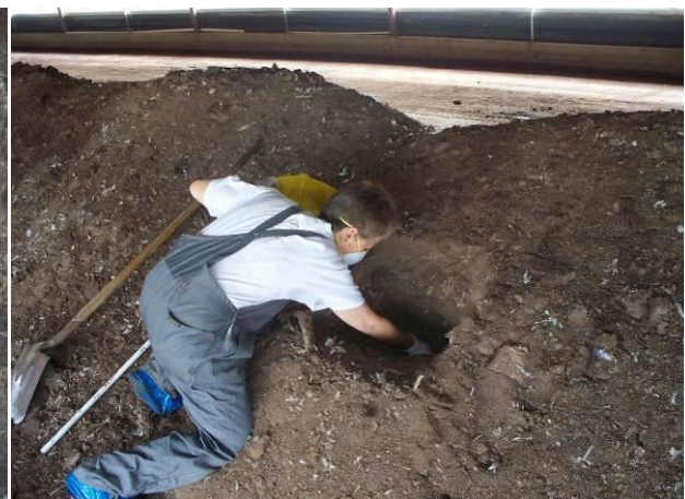
Figure 1-9: Sampling litter from a windrow at 25 cm depth.
