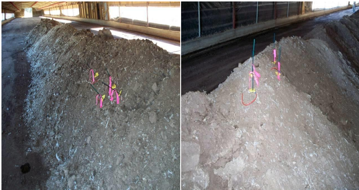
Figure 4-2: Windrow formation and placement of iButtons® in the windrow with bamboo stakes and ribbons as markers
