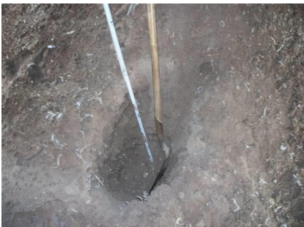
Figure 1-8: Sampling litter in a windrow with a depth marker.
