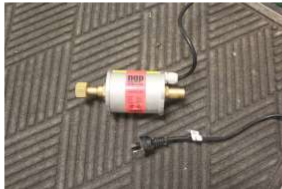
Photograph 10: CO 2 In-Line Heater Unit
